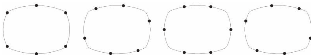
Fig. 7. Cases of joint location of segmental tunnel lining (compiled by authors)
