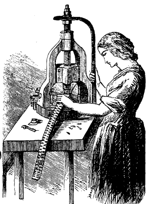
PEN MAKING—STAMPING PEN FROM STEEL.
