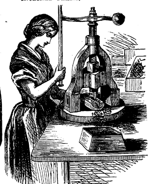
PEN MAKING—BENDING THE PEN.
